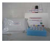
ELISA kit for determining milk progesterone
